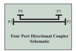
For the purpose of this analysis if P1 is the power incident at Port 1 then the output powers at Ports 2, 3 and 4 are P2, P3 and P4 respectively. If P2' is the power incident at Port 2 then P1', P3' and P4' are the output powers at Ports 1, 3 and 4 respectively.
