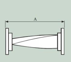
ORDERING INFORMATION Model: angle of twist, LH (left hand) or RH (right hand); description Example: Model 22450-90LH 90° left hand waveguide twist
