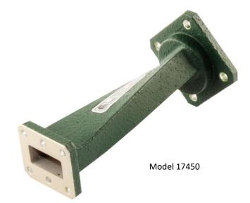
Flann Twists are manufactured from sections of standard waveguide which have been precisely twisted whilst maintaining the internal waveguide dimensions. Standard models are 90° left hand twists. Other configurations are available to special order, including:
