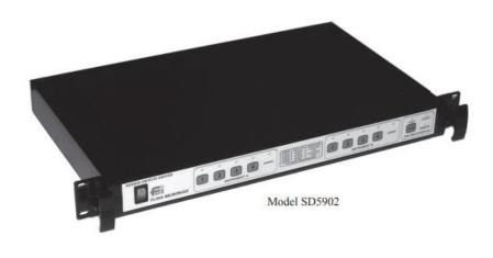
The Series SD5902 Waveguide Switch Driver is designed to control the Flann microwave range of Series 333-\*E Precision Waveguide Switches. It provides the interface between an IEEE 488 Bus (GPIB) or Universal Serial Bus (USB) and Precision Waveguide Switches and allows for manual operation with display of current status. The SD5902 will drive either a 2channel or a 3-channel switch without the need to reconfigure.
